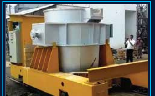
▲ Selfprimed Ladle Car Developed & Supplied for Molten Iron Transfer
