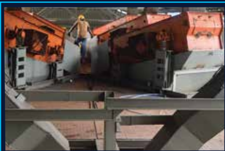
▲ Vibratory Feeders Developed In-House & Supplied to Pallet Plant
