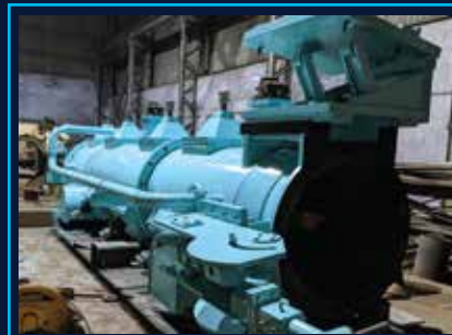
▲ 1st time in India we have designed Centrifugal casting Machine for Manufacturing of Ductile Iron pipes
