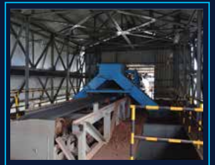
▲ Tripper Conveyor Developed In-House & Supplied
